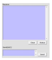
The "receive window" will show the message received from HD808. When you click the Control Buttons (Fig. see step 4) or send Control Command (Fig. see 2.3) to HD808, it will send out the message about "operation results" as below:
