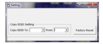
To click the menu to choose the INPUT A and Output B can copy the EDID of Output B Display to the Input A and also can do save of the EDID info . Factory Reset button represents the functions of setting the EDID back to the default EDID.(1080 2CH)
